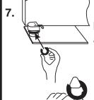
Using shims furnished with bottom arm, fill gap between arm and base.
