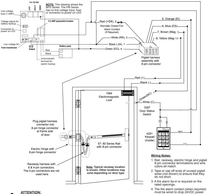
Electrified Trim applications require a separate raceway & power transfer device. Installation of conductors or harnesses (by others) through the exit device rail is prohibited as it could lead to product performance issues up to and including product failure.
