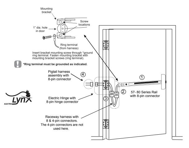
Note: No field rail cutoff allowed. Exit device must be ordered for specific door width.
