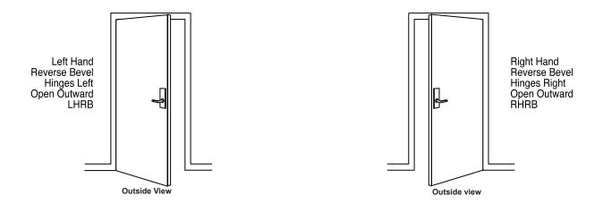
On inside of door, exit devices are oriented as follows:
