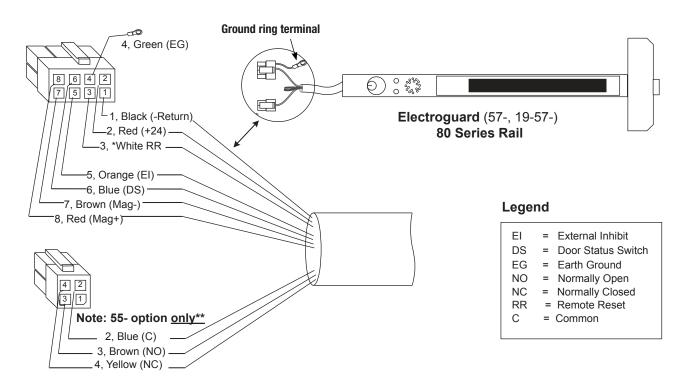
\* Note: White wire on previous Legacy product was used as Fire Alarm input option and has been replaced with RR.
