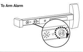
Turning key clockwise, the yellow PASSAGE LED will flash for 15 seconds (default), then a quick chirp and the ARMED green LED will flash and repeat every 30 seconds. Signal above cylinder indicates unit is armed.
