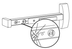
Horn chirps intermittently to indicate low battery condition. Change battery.
