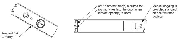
\*Field cut rail assemblies are not allowed. Exit Device must be ordered from the factory for specific door width.
