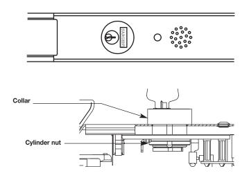
Side View. Battery holder not shown. Use caution not to damage wires when installing cylinder nut.
