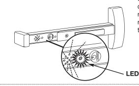
When ARMED, depressing the push rail will activate the alarm and the horn will sound and red violation LED flashes. The horn will continue to sound for 2 minutes (default). After 2 minutes the unit will reset on its own and the red LED will flash every 30 seconds until rearmed using the key. Turn the key counter clockwise to deactivate the alarm, then clockwise to rearm.
