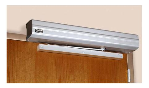
The Norton 5700 Series low energy operator is designed for quick install and consists of three basic components: inverter, motor, and Norton's 5700 closer body.
