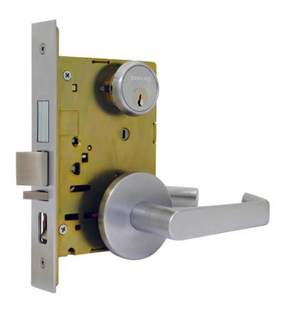
The SARGENT 7900 series Mortise Lock, is an ANSI/BHMA A156.13 Series 1000 Grade 1 mechanical mortise lock. It has a reversible stainless steel latch, independent non-handed stainless steel deadlatch.
