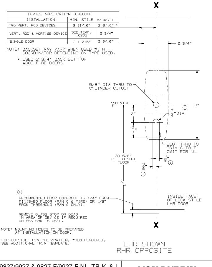
CX9827/9927 & 9827-F/9927-F NL, TP, K, & L Series Vertical Rod Device (Wood Door)
