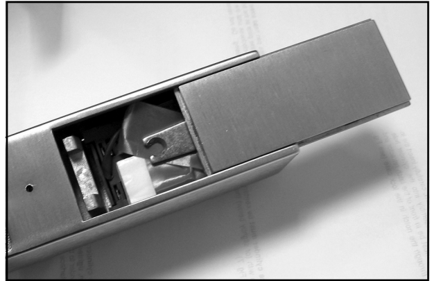
Fig. 7a: Install the battery pack: Push all wires inside the battery compartment and slide plate back on.
