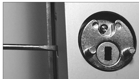
Fig. 5d: Tighten the interface cylinder set screw
